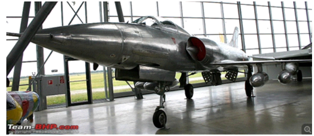
This photo shows - Marut's streamlined, aerodynamically clean pencil fuselage with its side air in-takes for the twin power plants; thin wing designed for supersonic flight; wide track under carriage to support landings on rough airfields; the bubble canopy for good visibility. Photo Copyright: Kurt Tank
